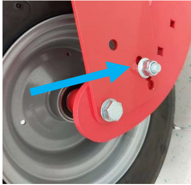
Figure 4: Installation on the second hole from the top with the nut on the outside
