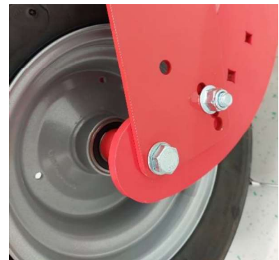
Figure 3: Harrow installed on the feeler wheel
