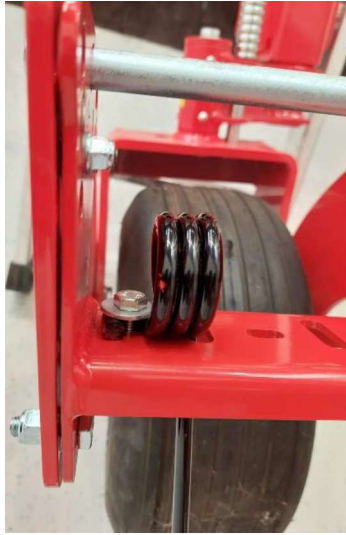
Figure 8: Tine fastening on the feeler wheel harrow 1
