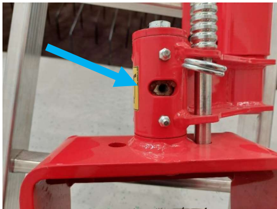
Figure 6: Thread on the pivot joint of the section
