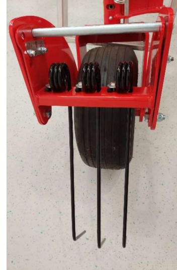
Figure 10: Tine fastening on the feeler wheel harrow 3
