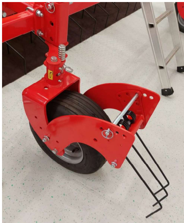
Figure 11: Completely installed feeler wheel harrow
