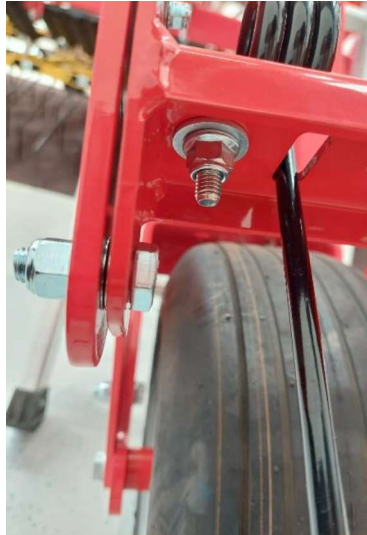
Figure 9: Tine fastening on the feeler wheel harrow 2
