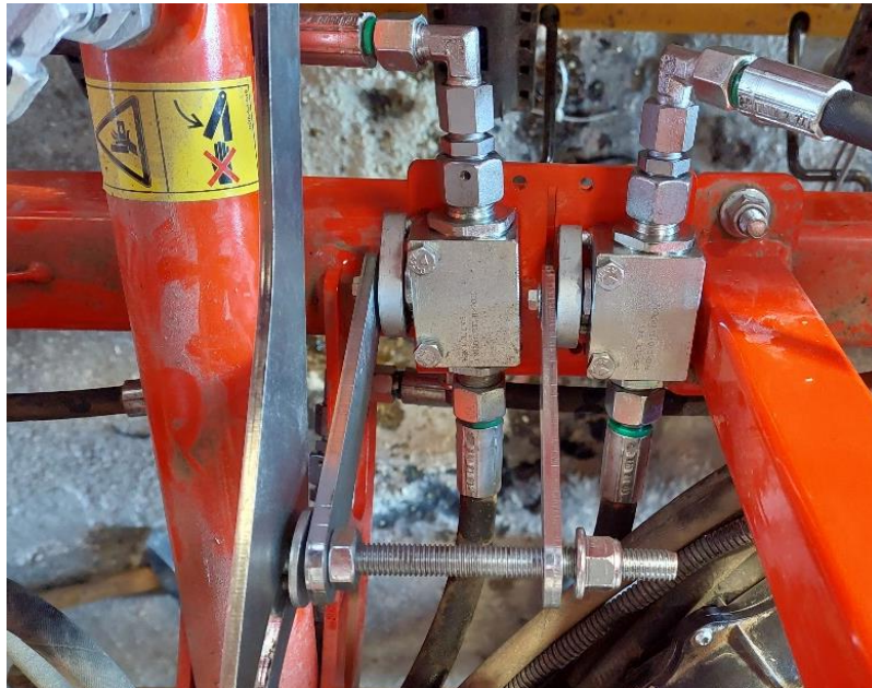
Figure 30: Control linkage connected to the stroke limiters
