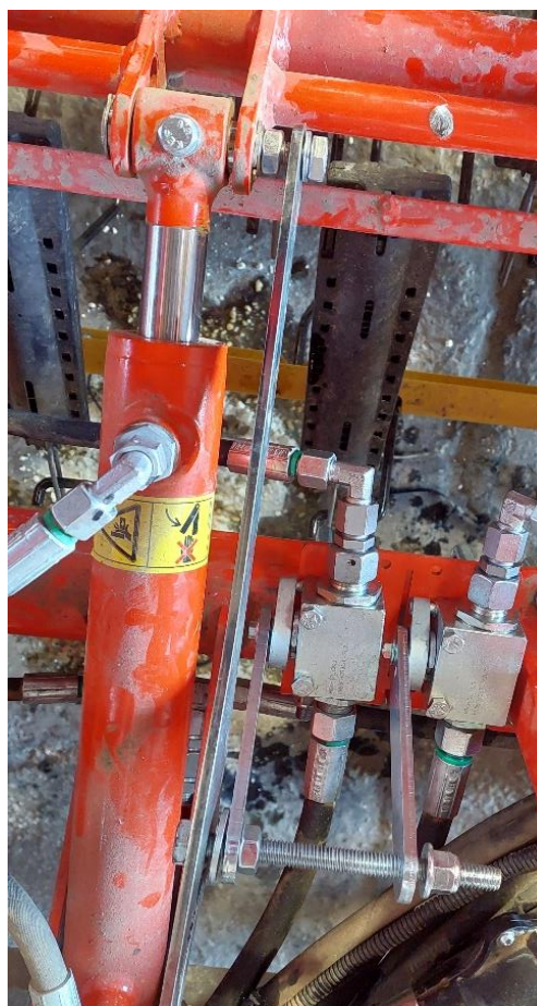
Figure 31: Completely installed control linkage
