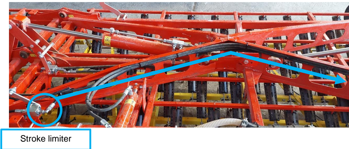
Figure 16: Hose laying from the stroke limiter to the flow divider 1
