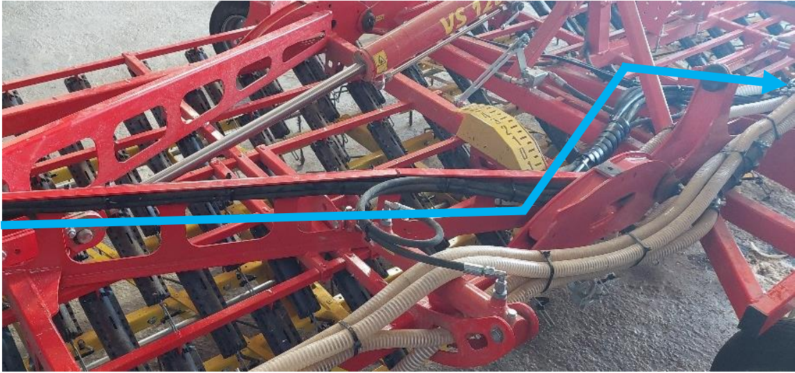
Figure 17: Hose laying from the stroke limiter to the flow divider 2
