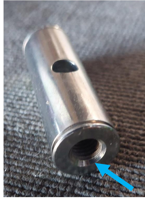
Figure 28: New pin with internal thread
