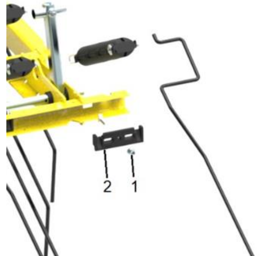
Figure 18: 1 = nut, 2 = plastic part
