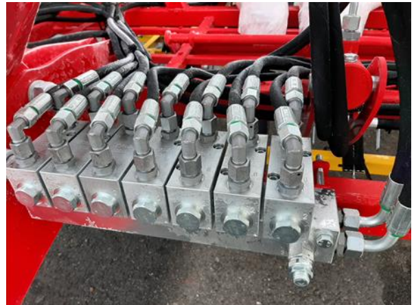
Figure 14: Flow divider on the center frame
