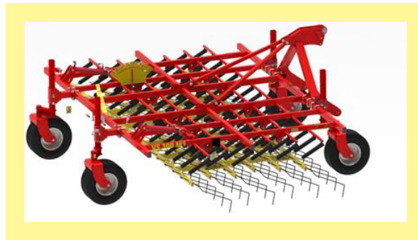
Figure 11: Front mounting with 4 feeler wheels
