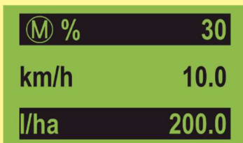
Figure 5: Work screen without speed sensor
